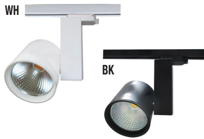
▲ 8356-30K LED TRACK LIGHT Die-Casting Aluminium Body 40W LED, 4500Lm, T. Color: 3000K Beam Angle 28° 90-305V / 50-60Hz Size: D-125mm Available in: Matt White, Matt Black
