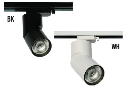
▲ 8789-30K LED TRACK LIGHT Die-Casting Aluminium Body 20W LED, 2000Lm, T. Color: 3000K Beam Angle 36° 100-277V / 50-60Hz Size: D-78mm H-230mm Available in: Matt White, Matt Black
