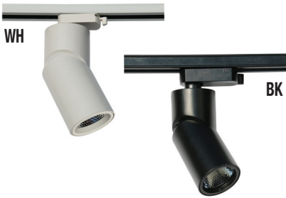
▲ 8788-30K LED TRACK LIGHT Die-Casting Aluminium Body 7W LED, 700Lm, T. Color: 3000K 100-277V, 50-60Hz Beam Angle 36° Size: D-56mm H-180mm Available in: Matt White, Matt Black
